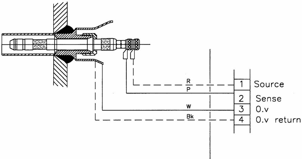
**Fig. 4.1b Probe Normally in Water.
