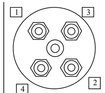
Set torque wrench to 25Nm and tweak each nut until the wrench clicks at the torque limit.
