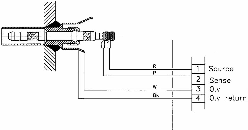
**Fig. 4.1a Probe Normally in Steam.
