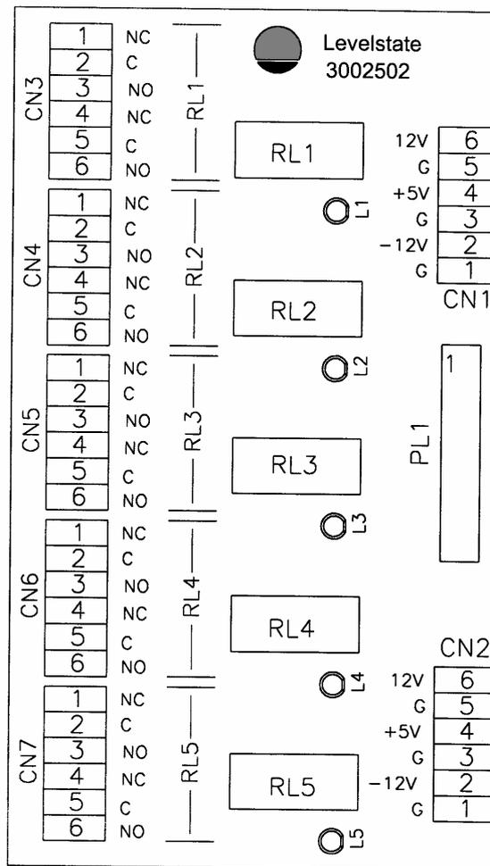
**Fig. 2.4 ELS 300 Relay PCB**
