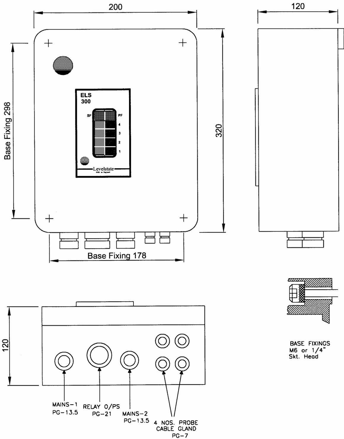
**Fig. 2.2 Electronic Unit Dimensions And Cable Gland Location**
