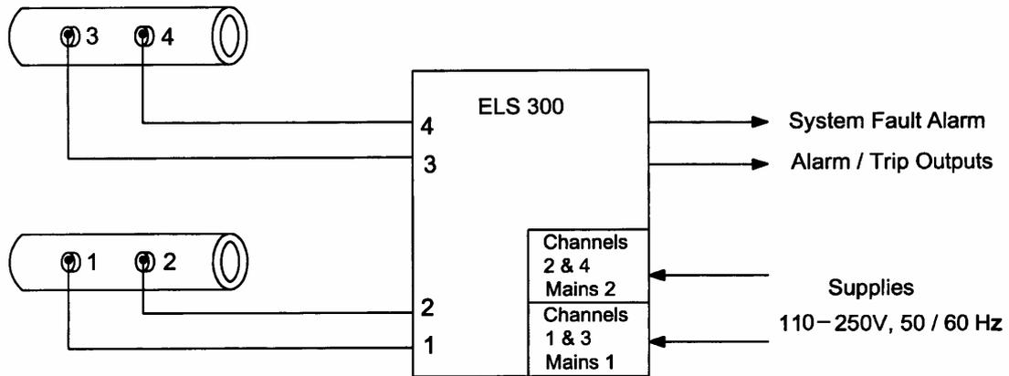
**Fig. 2.1a Coincident Probe Configuration**
