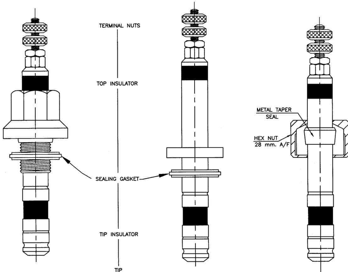
**Fig. 3.0 Standard Probes For ELS 300**
